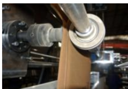
side ultrasonic sealing of tshirt bag
